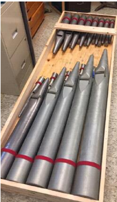
Crated pipes ready for shipping to Ohio for refurbishing. Note the badly rusted tuners at the bottom right of the photograph. These will be replaced with new slider/tuners.
